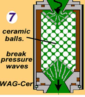
SELECTION is simply by connection, unless our associate LIQUID DYNAMICS International has completed an acoustic model study for you. (5) WAVEGUARD HO , uses the Helmholtz Orifice technology for greater efficiency for size. (6) Is for particulate laden systems, & is larger. (7) Is for the ultimate acoustic performance.
